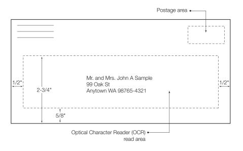
2.2 Address Placement Causing Mail to be Nonmailable or Nonmachinable The location of the delivery address on a letter-size mailpiece determines which dimensions are the length and height of the piece. Consequently, the placement of the address may render a piece nonmailable or nonmachinable.
